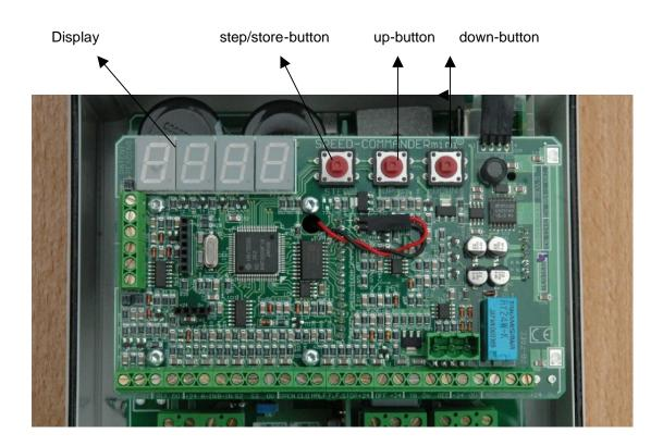
The encoder gives off pulses per rotation of the motor. The control counts these pulses and accordingly determines the position of the door. To do this, the control needs to be pre-programmed with what to do with each number of pulses.
